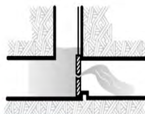
Cracked Gate Leaf
